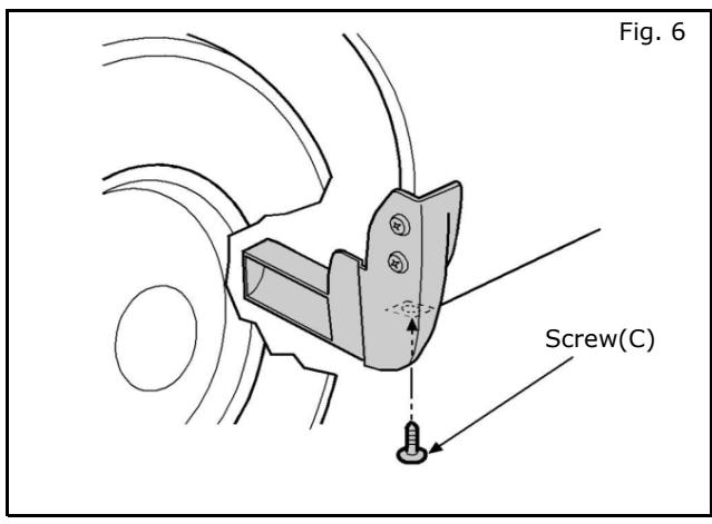
8) Align lower hole in Splash Guard to lower hole in fender and loosely attach Splash Guard to fender using Screw(C).
