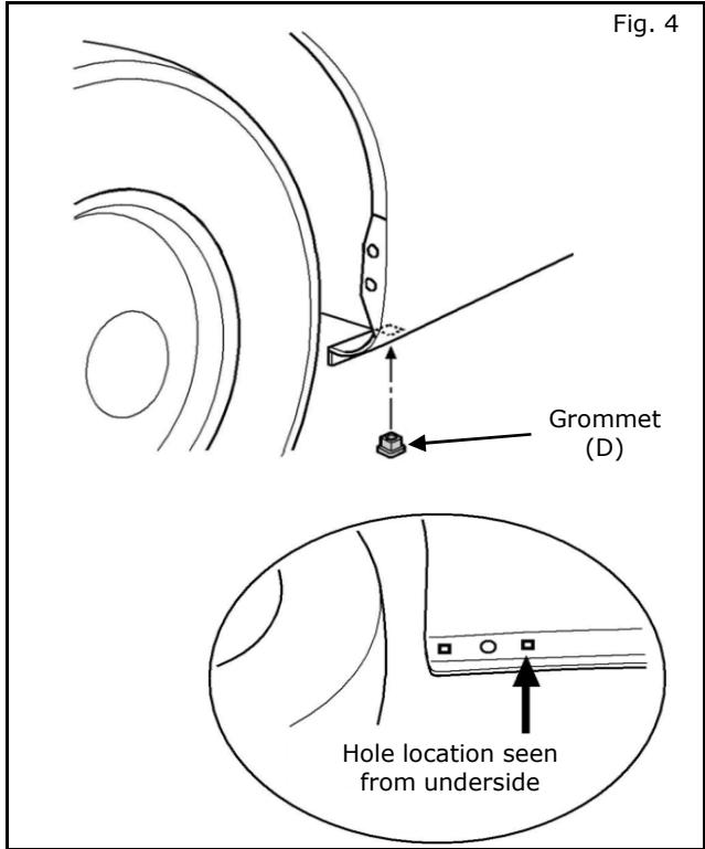
6) Insert one Grommet (D) into rear most square hole.
