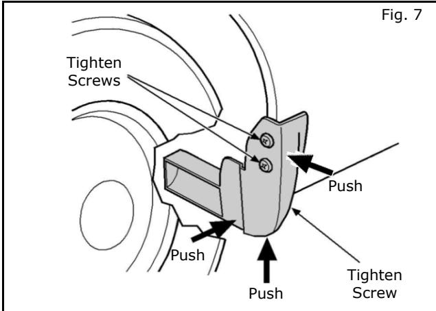
9) Push Splash Guard up, inboard and rearward firmly to fender to ensure there is no gap around the Splash Guard and tighten all screws shown.
