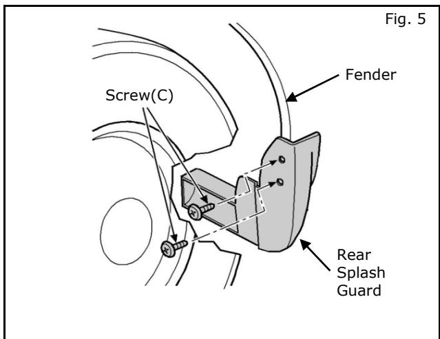
7) Align two holes in Splash Guard to two holes in wheel liner and loosely attach Splash Guard to wheel liner and fender using Screws(C).
